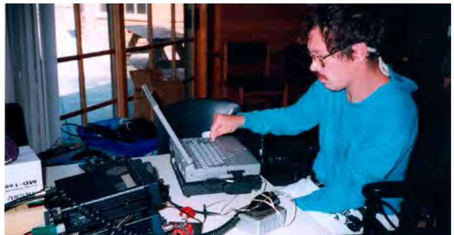
Rick Jorgenson, KBØQPY, in Rhode Island, uses a Pentium Laptop to generate voice output. Note the Rig’s microphone attached to the computer speaker.
